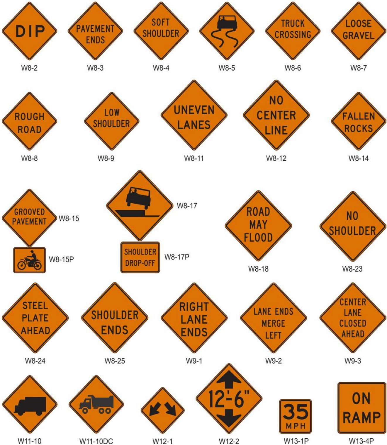
Figure 6F-4. Warning Signs and Plaques in Temporary Traffic Control Zones (Sheet 2 of 3)
