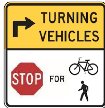
Figure 39 | R10-15R (mod) Stop for Ped-Bike Sign
