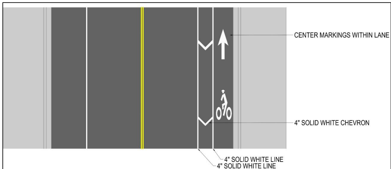
Figure 16 | Buffered Bicycle Lanes (Along Curb)
