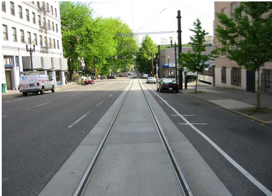
Figure 5-11 | Embedded Track Slab
