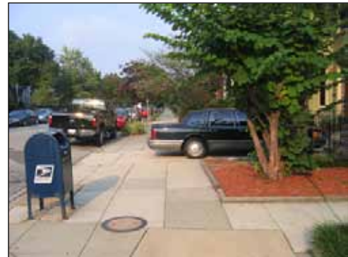
Example of a short driveway that cannot accommodate a typical vehicle without blocking the sidewalk
