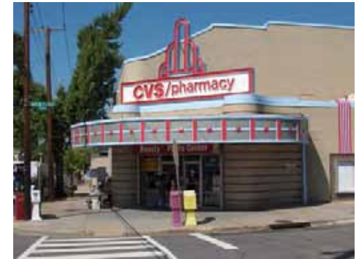
Marquees in commercial or industrial areas may extend up to 5 feet into public space.
