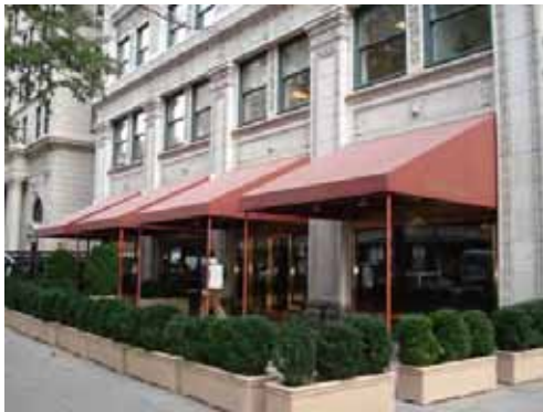
Planters – including vegetation – around a sidewalk shall not be higher than 36 inches.
