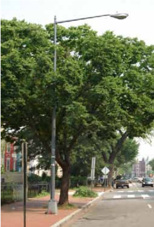
Street trees must be planted no closer than 15 feet from a light pole.
