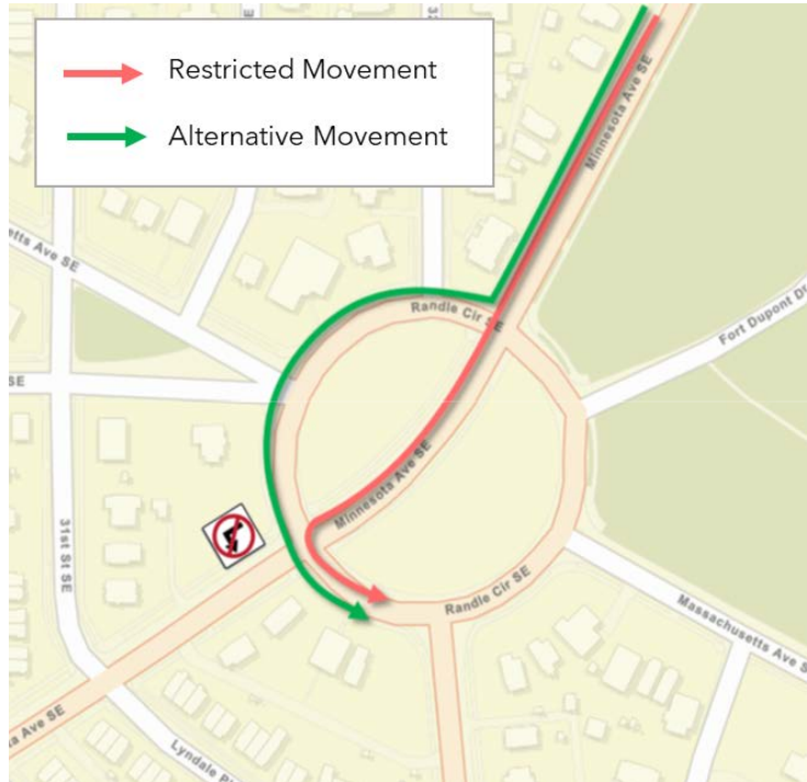
Figure 5: Illustration of restricted movement and alternative movement resulting from left turn prohibition.
